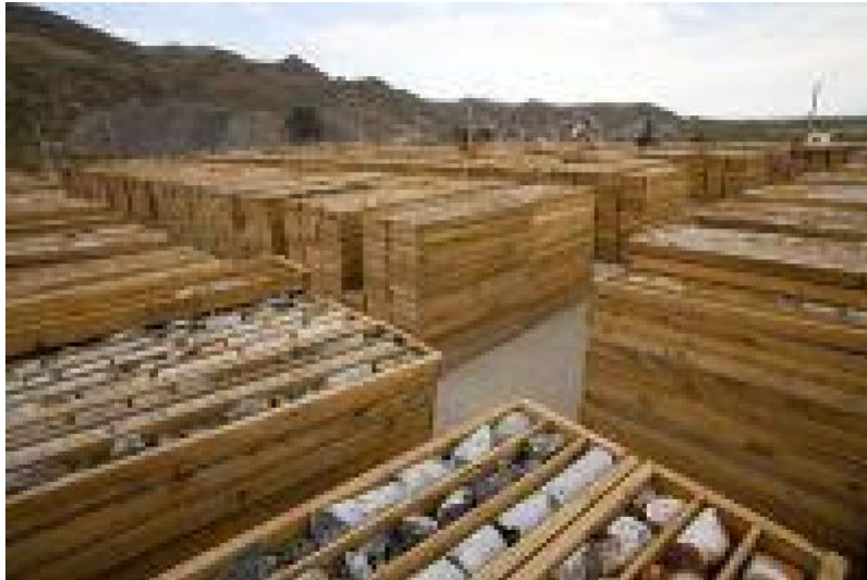
Bohrkerne; Foto: Excellon Resources
